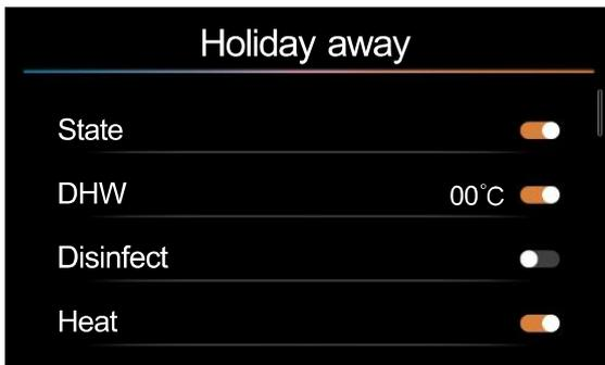
On the Holiday away page, Select DHW and press the [ < ] or [ > ] to set On/Off. On the Holiday away page, Select DHW and press the [ ○ ] to activate setting temp, if DHW is On.
