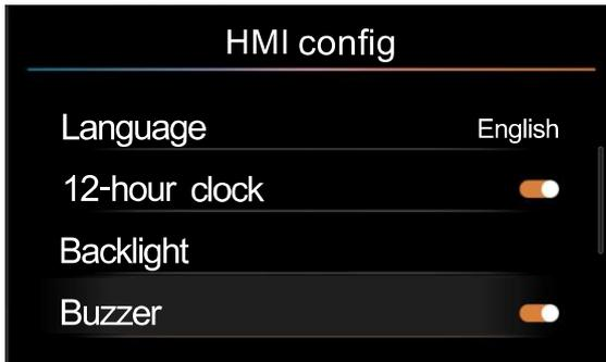
On the HMI config page, select Buzzer and press the [ < ] or [ > ] to set On/Off.
