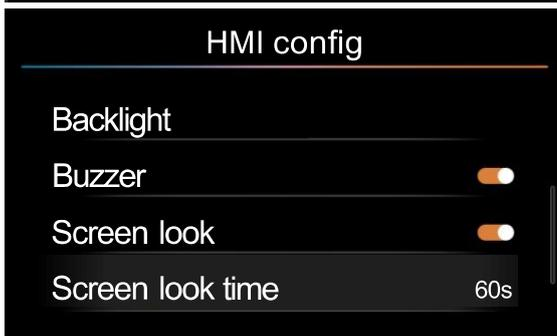
On the HMI config page, select Screen lock and press the [ < ] or [ > ] to set On/Off. On the HMI Config page, select Screen lock time and press the [ < ] or [ > ] to set the time. The time range is 10-120s (default 60s).
