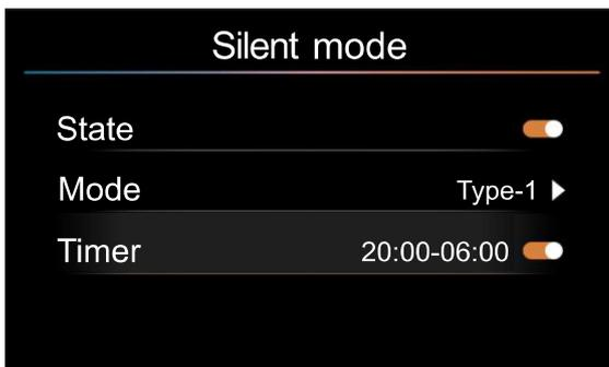
On the Silent mode page, select Timer and press the [ < ] or [ > ] to set On/Off. When set Timer off, the unit operates in Silent mode all the way. By pressing [ ○ ] and pressing the [ < ] or [ > ] to select hour/minute of the start time and hour/minute of the end time, you can change time.
