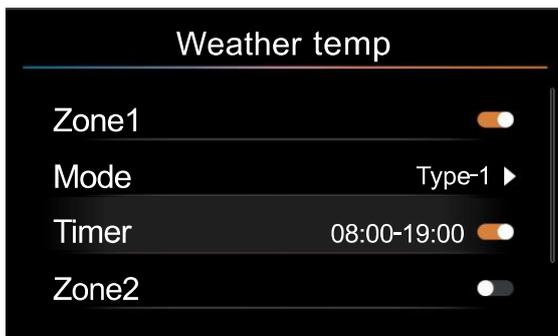
On the Weather Temp page, select Timer and press the [ < ] or [ > ] to set On/Off.
