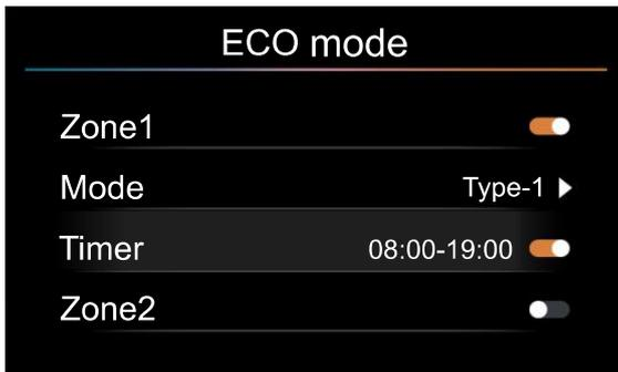
On the ECO mode page, select Timer and press the [ < ] or [ > ] to set On/Off. When set Timer off, the unit operates in ECO mode all the way. By pressing [ ○ ] and pressing the [ < ] or [ > ] to select hour/minute of the start time and hour/minute of the end time, you can change time.
