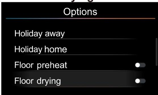
On the options page, select Floor drying and press the [ < ] or [ > ] to set On/Off.
