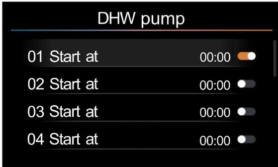
Select Start at and Press the [ ] to active start time setting, then press the [ ] or [ ] to select hour/minute, and press the [ ] or [ ] to change the clock number.
