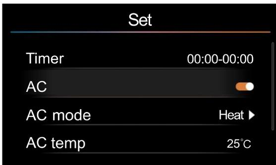
On the Set page, select AC and Press the [ ] or [ ] to set On/Off. On the Set page, select AC mode and Press the [ ] or [ ] to select AC mode according to the following order: Heat→Cool→Heat. On the Set page, select AC temp and Press the [ ] or [ ] to set temperature.
