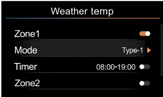
On the Weather Temp page, Select MODE and press the [ < ] or [ > ] to select the different level according to the following order: TYPE-1→TYPE-2→TYPE-3→TYPE-4→TYPE-5→TYPE-6→TYPE-7→TYPE-8→Custom→TYPE-1.
