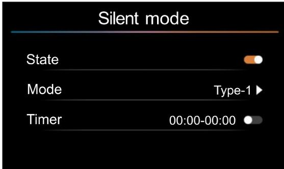
On the Silent mode page, select Mode and press the [ < ] or [ > ] to select the different level according to the following order: TYPE-1→TYPE-2→TYPE-1.
