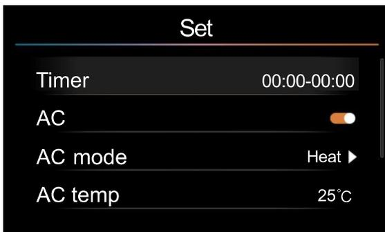
On the Set page, select Timer and press the [ ] to set the start and end time. Press the [ ] or [ ] to select hour/minute, and the [ ] or [ ] to set the time.
