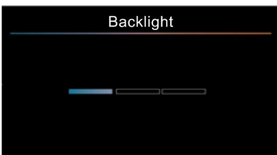
On the HMI config page, select Backlight and press the [ o ] to enter the Backlight page. On the Backlight page, press the [ < ] or [ > ] to set screen brightness
