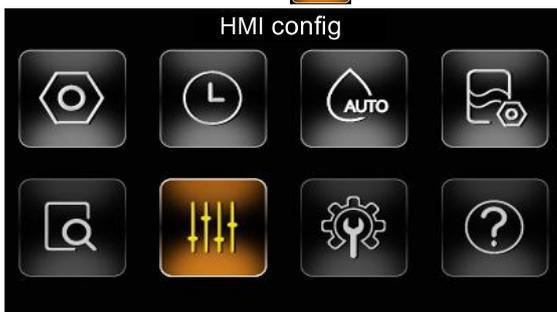
On the Menu page, select HMI config and press the [
