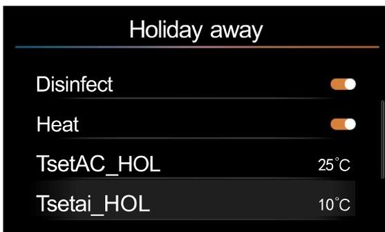
On the Holiday away page, TsetAC\_HOL means setting water temperature, and Tsetai\_HOL means setting room temperature. Select TsetAC\_HOL and press [ < ] or [ > ] to set temp. Select Tsetai\_HOL and press [ < ] or [ > ] to set temp.
