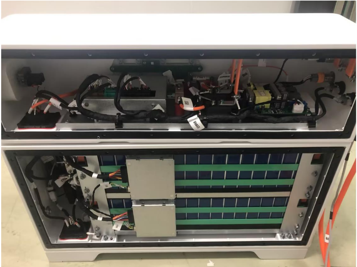
Internal View of Battery Module
