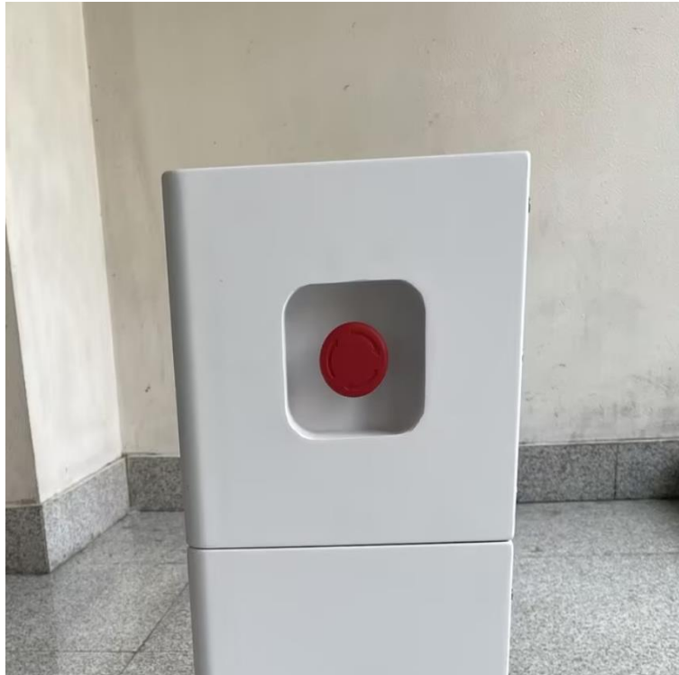
Overall External Side View of High-voltage Box
